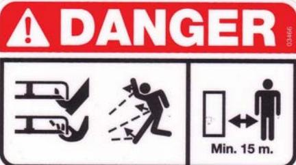
**WARNING!** SHARP PARTS. Keep hands and feet away. Do not operate the mower over gravel or foreign bodies which may be sucked up and ejected by the blades, generating a danger. Keep people at a min. distance of 15 metres. Remove the key and read the instruction manual before attempting to carry out any maintenance or repairs to the machine.
