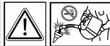
Handle fuel with care, it is highly flammable: Do not refuel machine while smoking, when machine is near an open flame or sparks, or when the engine is running. Stop the engine.
