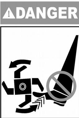
**WARNING! SHARP PARTS.** Keep hands and feet away. Do not operate the mower over gravel or foreign bodies which may be sucked up and ejected by the blades, generating a danger. Keep people away. Remove the key and read the instruction manual before attempting to carry out any maintenance or repairs to the machine.
